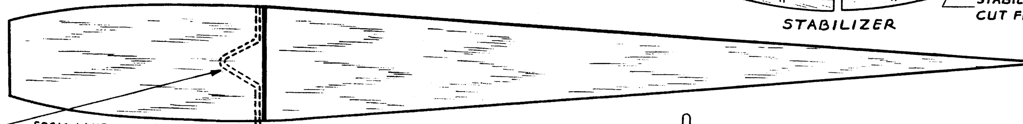
FUSELAGE BOTTOM VIEW CUT FROM 1/16 SHEET Balsa
