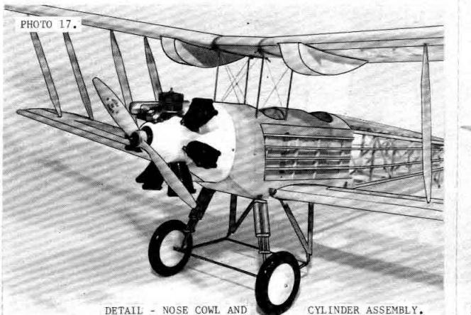
DETAIL - NOSE COWL AND CYLINDER ASSEMBLY.
