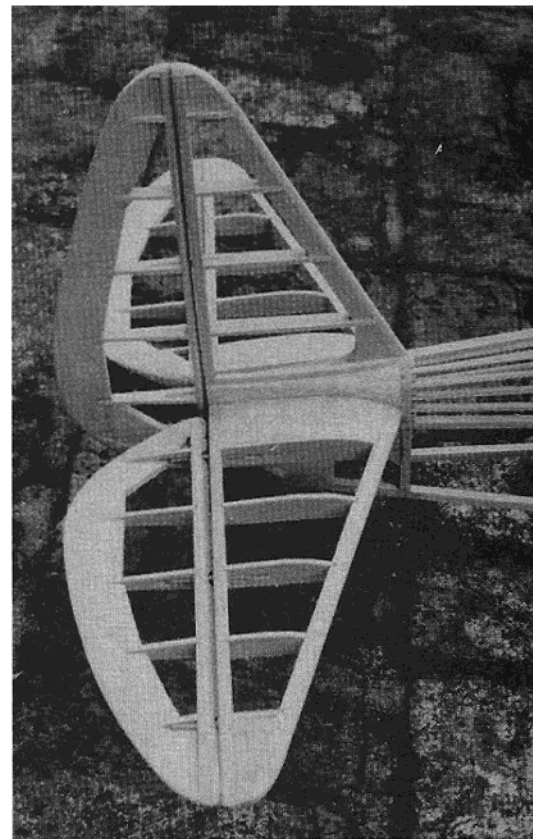
Tailplane detail showing block fill and counter-boring for hinge points. Note the points visible within the ribs.
