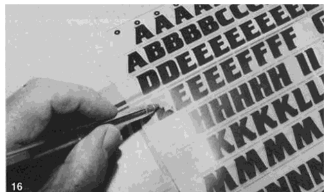
Decorative trim was from two thicknesses of black chart tape available from artists' stores (14). Fuelproof afterwards. Name was applied by Letraset, pre-release letter by rubbing onto backing sheet (15). Transfer to wing and lightly press into place (16 & 17).
