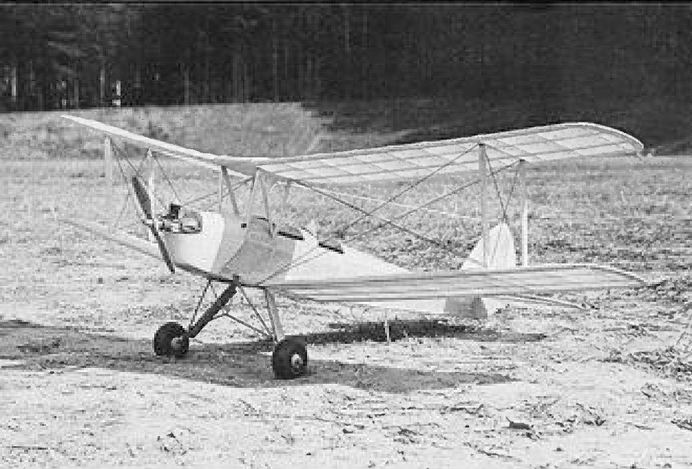
Note landing gear suspension system. Wing rigging is functional.
