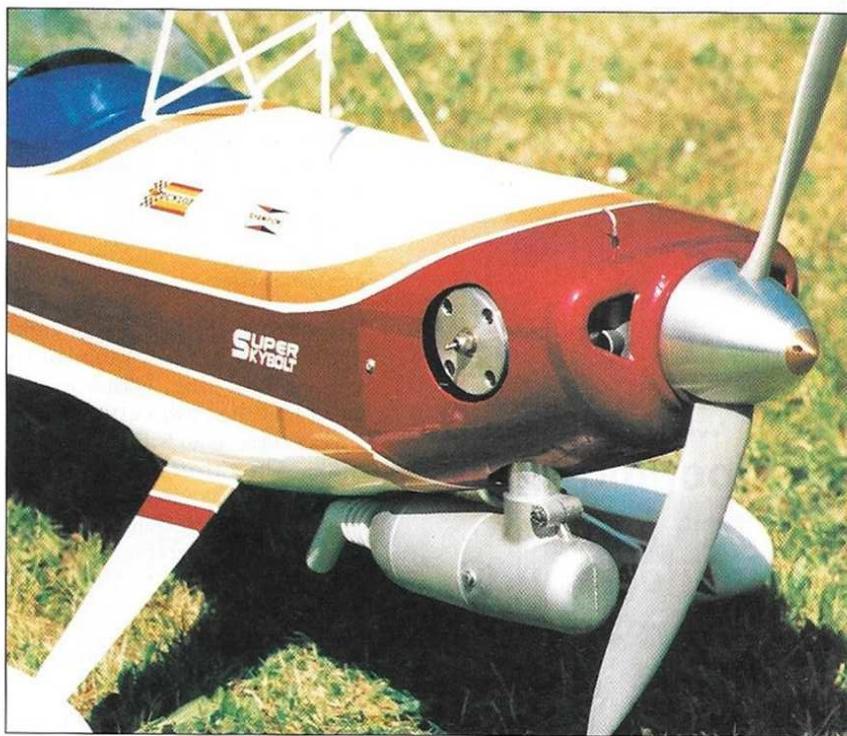
Above: Neat engine installation. Gordon will fit a finned head for better cooling.
