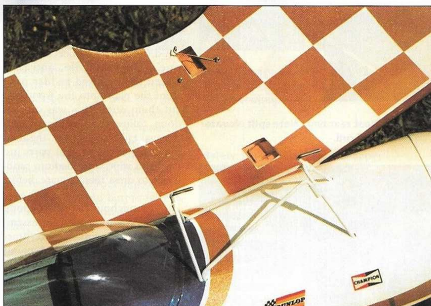
Above: Cabane-wing fix; wire prongs engage in tubes within the centre section.
