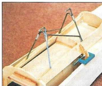
Cabane mounted on the fuselage. Clamp is holding spruce reinforcing strip while glue sets. Gusseting between cabane mount and cockpit floor is still to be added.
