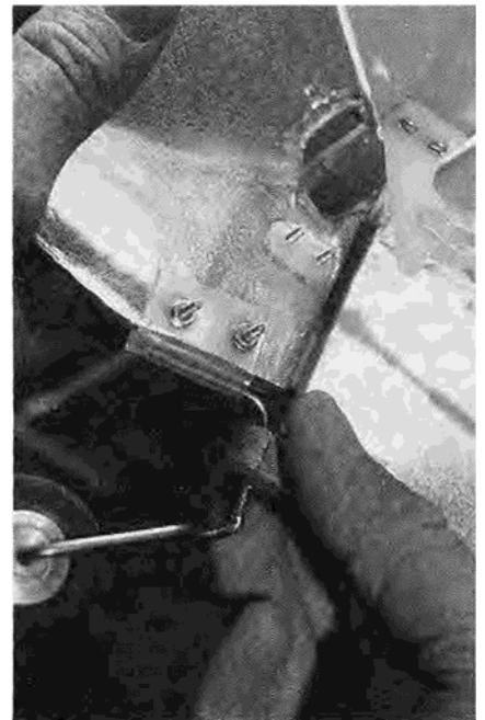
A sleeve of plastic cut from a six-pack ring makes a simple, shock absorbing sleeve for the tail wheel tiller. Like the rest of the model: somewhat crude --- but effective!
