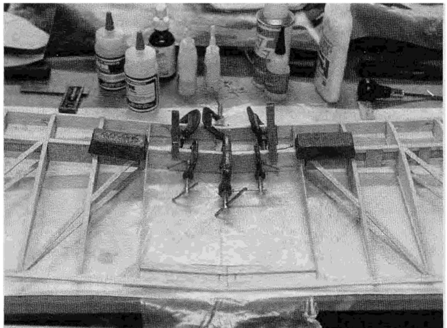
With weights and brads holding the halves in alignment, the wing panels are joined using slow setting epoxy and 1/16" plywood dihedral gussets.
