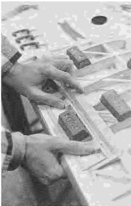
Brass rods with little dabs of paint on their ends are put into the hinge holes in the aileron and slid into place against the wing, thus marking the exact position of the hinges on the rear spar prior to drilling.
