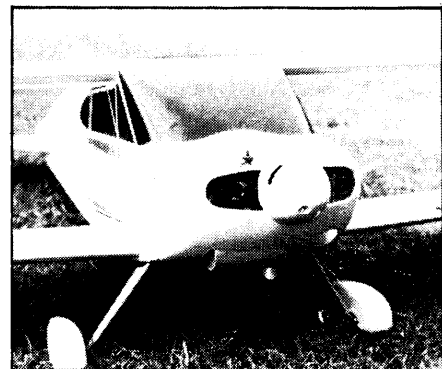
Wheel spats can be fabricated from balsawood and plywood or from glassfibre. Ailerons are fitted to the top wing only although the full size aircraft uses 'flaperons' on both wings.
