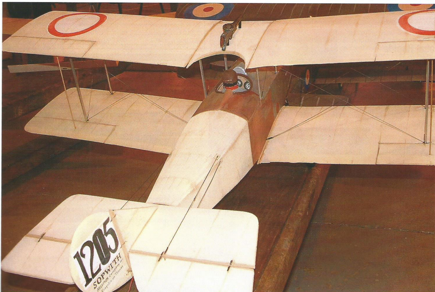
This 35" span version of the SS3 was my first 'foamie' and was really just a bit too big and heavy for a GWS A series IPS and seven little NiCads, but when re-motored with a GWS twin IPS and an 1147 prop it flew really well.
