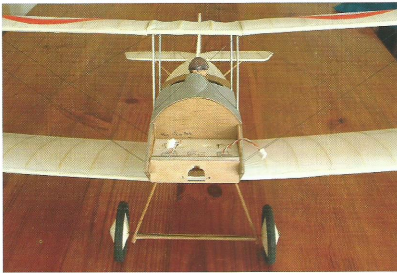
LEFT: Coming along nicely; the Falcon PU01 motor just screws to F1. You can add side-thrust with a bit of packing. Spot the mistake on the centre-section covering - it should be cut across the grain like the wings, then it would not sag so much between the ribs.
