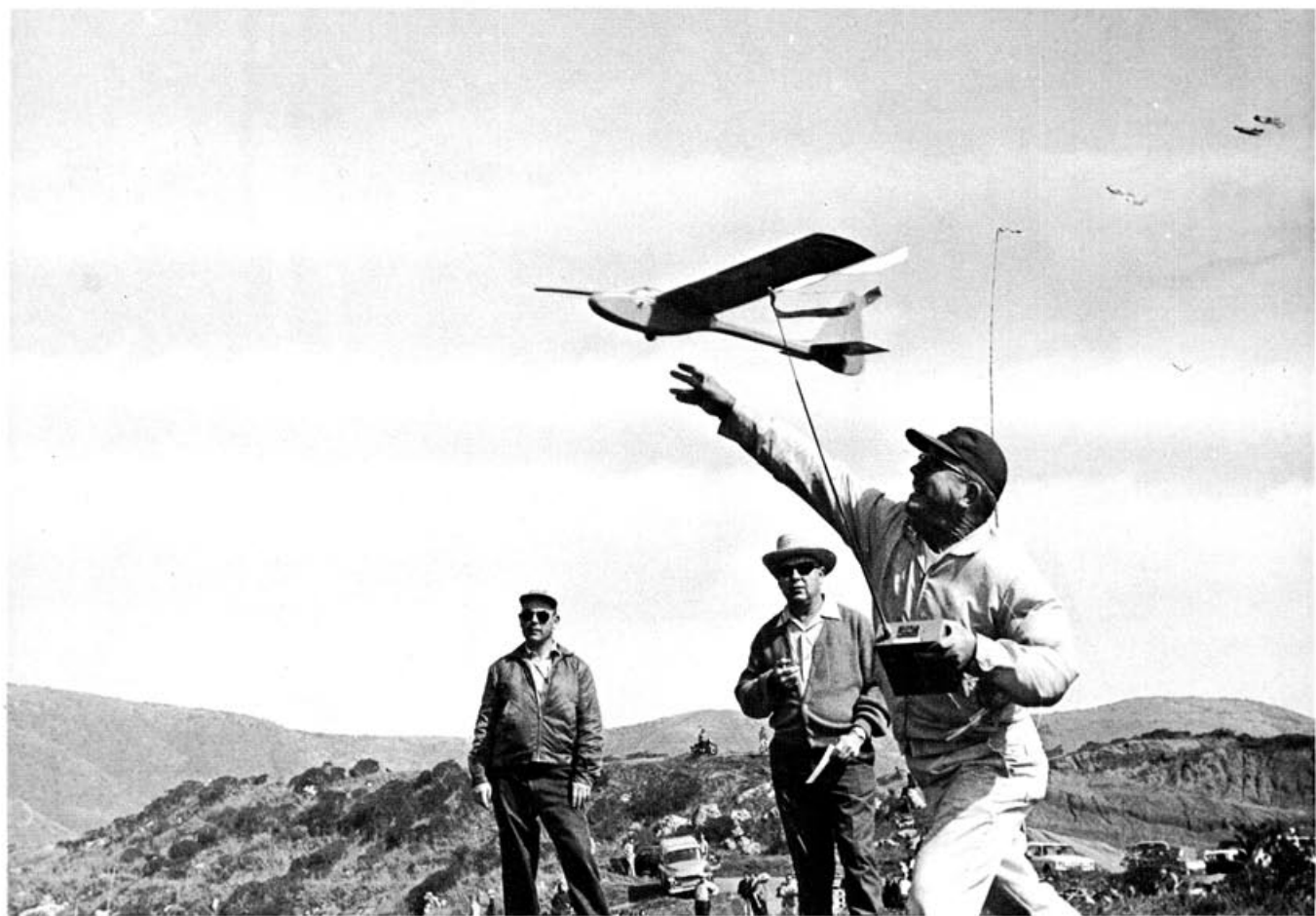
The Slopemaster about to capture second place in its first contest. Note stabilizer on top of boom — before modification. Note pot on Chief Sunday Flier. This picture also taken before he got streamlined!
