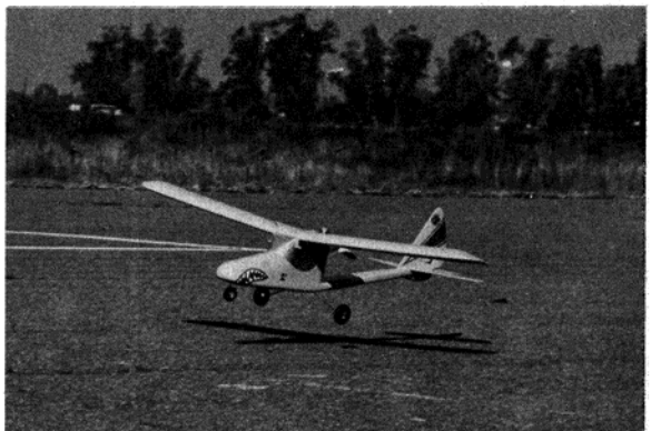
Gentle flair for landing. Wing with thick airfoil provides excellent low speed characteristics.
