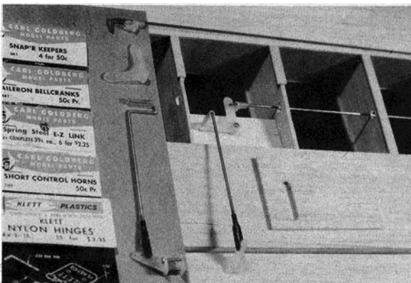
Aileron control parts and installation. Pushrod from bellcrank to horn can be removed for wing covering and reinstalled.
