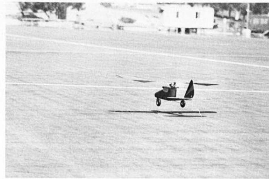
At left, the .049 powered RCM Scooter takes off for another flight. Takes off quickly on a smooth field, but can be easily hand-launched for cow pasture flying. Any Cox .049 engine works well.
