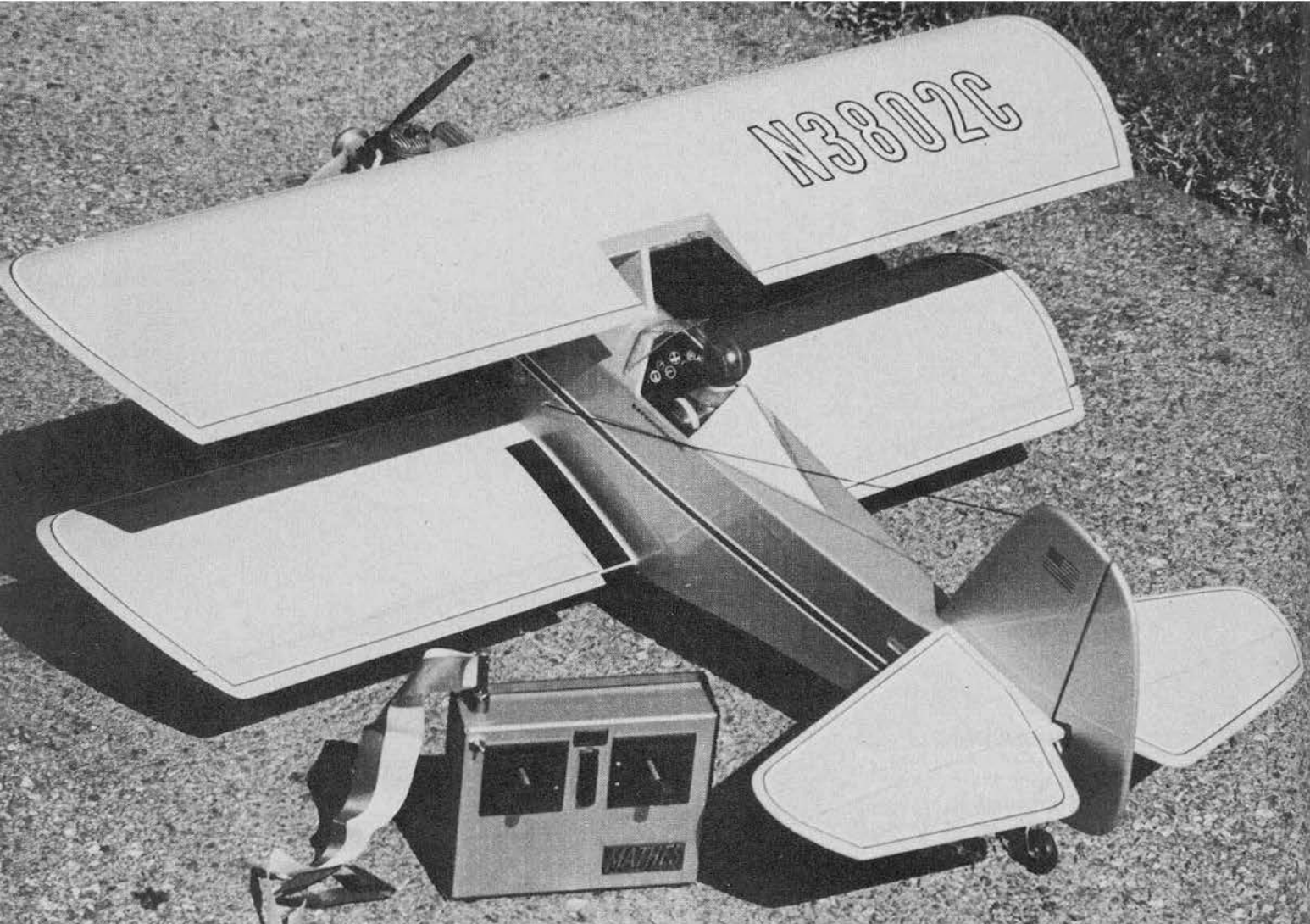
Don Dewey's version of the RCM Basic Biplane by John Chapis. Veco-Lee .19, Mathes Electronics radio. All-up weight, four pounds. If you like biplanes, but are not overly fond of cabane struts, the center crutch pylon used in the Basic Biplane solves the construction problems.
