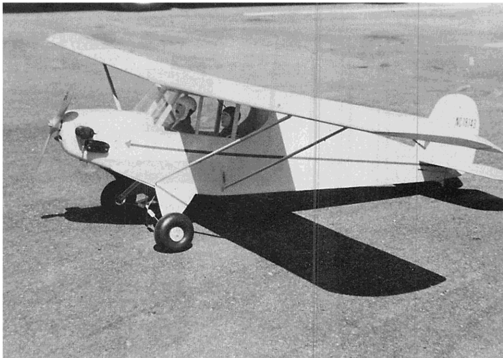
An ancient Super Tigre .51 still puts out more than enough horsepower. Uses a 3/4" K&B extension shaft. Cowling is from a Sig J-3 Cub. Tailwheel steering with horns is simple. At top: In flight, dead stick.
