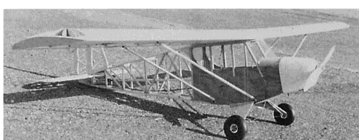
A few longerons, uprights, diagonals does it. Your radio will fit in easily. At left: Built up tail feathers. Framework is enough, light, well stressed.
