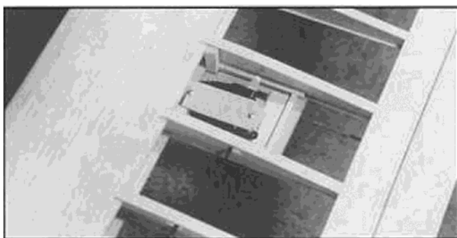
LEFT: Completed airframe; note the simple, straightforward construction throughout. ABOVE: Spoiler-aileron servo installation in wing.
