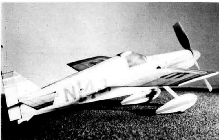
Windshield, cheeks, and wheel pants were molded on Mattel Vacu-Form on the original. Pants and cheeks can be carved from balsa.
