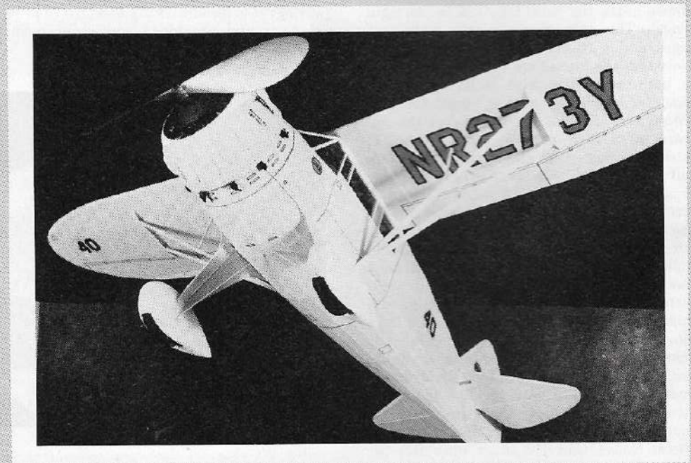
Underview of the Mulligan reveals detail of the wing struts, wing cuffs, and gear fairings. The registration number decal must be cut to clear the strut joint. Line details are done with a Rapidograph pen.
