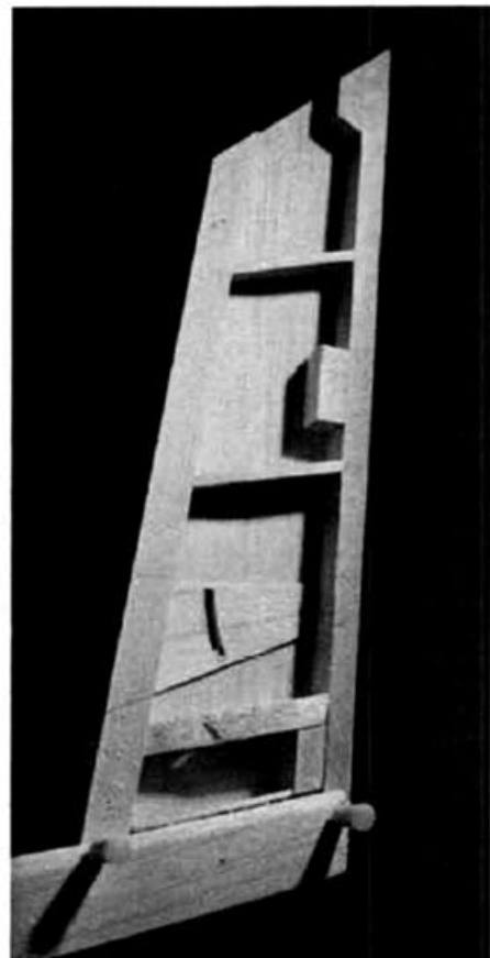
Fin sides are reinforced inside and outside with thin plywood where stab mounts. Firm! Small blocks are for hinge support.
