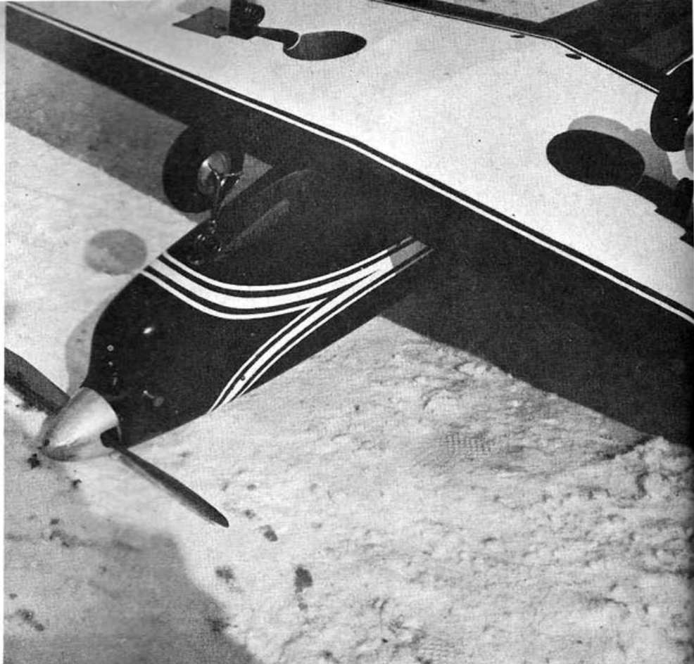
Main gear uses wheel well covers, nose gear wheel well is uncovered, needle valve is only projection in breeze when model is in full flight. Note Camlocs used to hold wing in place.
