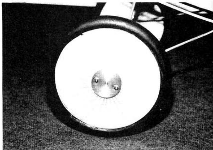
The outside of wheel. Note that holes for wires are not yet made in the hub plate.
