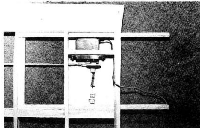
Close-up of aileron servo installation.
