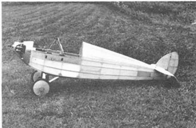
Baby Bullet's fuselage and tail group ready to be painted.
