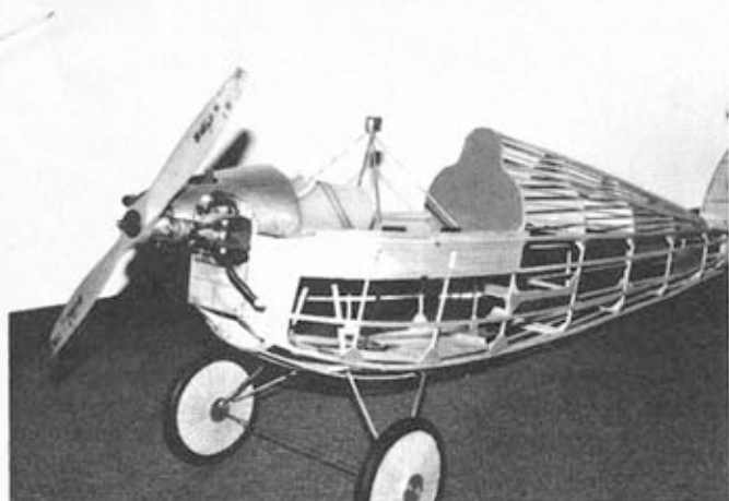
Heath Baby Bullet's fuselage ready for covering.
