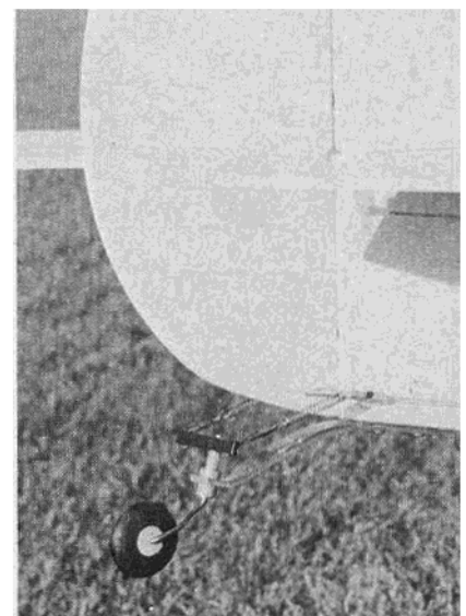
Built up tail wheel assembly.
