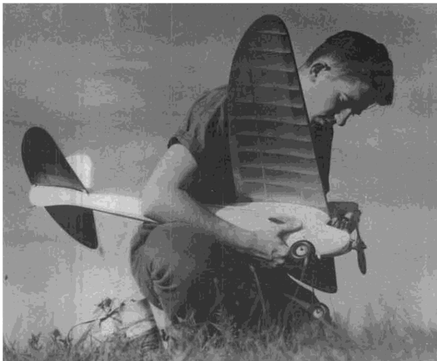
A youthful Carl Hermes with his Hayseed B, somewhere in Connecticut in 1941. Powerplant was an Ohlsson .23. Original color scheme was red, white, and blue; details on plan.
