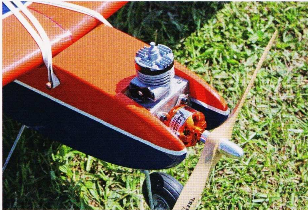
It's important to have bind free hinges and light but rigid pushrods when using a Galloping Ghost actuator.
