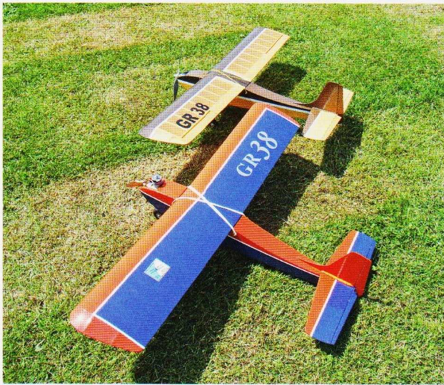
Gary's Australian built 3-channel model and Glyn's tissue covered version with additional ailerons.
