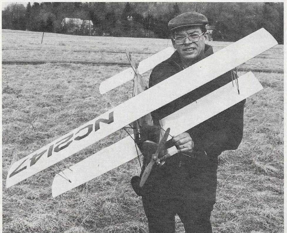
Some welding rods bend up to form the cabane struts, easily enough. The landing gear is routine. Below: Boxy in line perhaps, this due to its home-built heritage. Trexler wheels are a natural.
