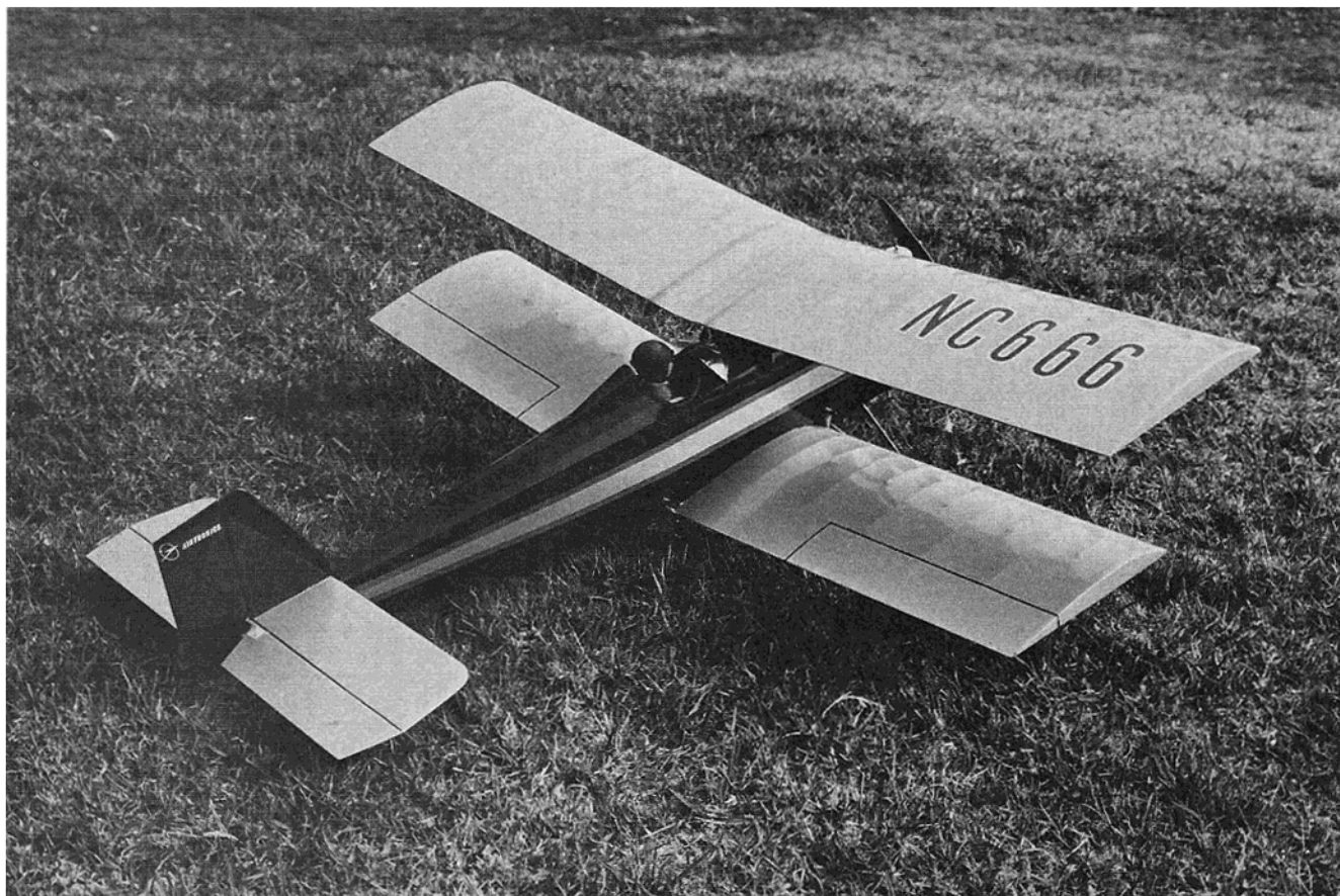
One of the Gere 3-channel prototypes, finished in black and silver Solarfilm. DJ's trim tape outlines dummy ailerons.
