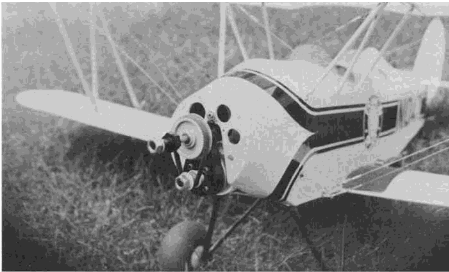
Installation details for the Astro Flight 15 motor with 10/15 speed reducer. Holes in forward bulkheads allow cooling air to flow through to battery. A 12v blower is used while charging.
