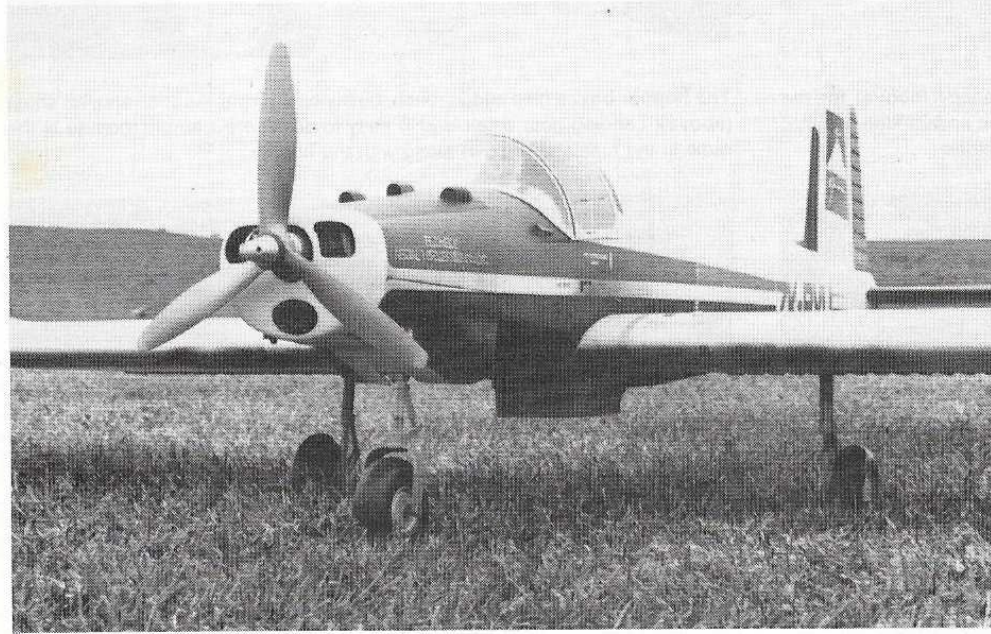
The aileron tip shape is achieved with the (above left) use of a carved balsa block. With the tail cone removed (above right), it's easy to see the lead-out for the antenna, and the internally actuated rudder. The three bladed prop (below) serves a dual purpose; static display and flying the plane.
