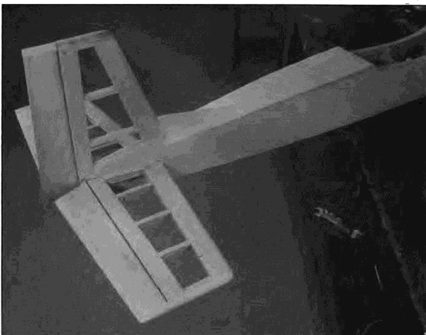
Assembled vertical fin and stabilizer fitted to fuselage. Hinge pins should be removable for access to elevator control horn.
