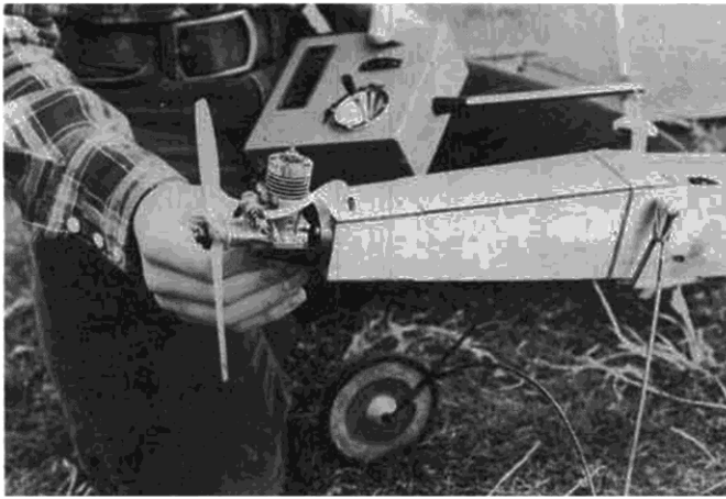
Brian McCleave adjusts the throttle linkage on his OS .10 powered Dragonfly. Kraft-Hayes mount. Imagine the fuel economy!
