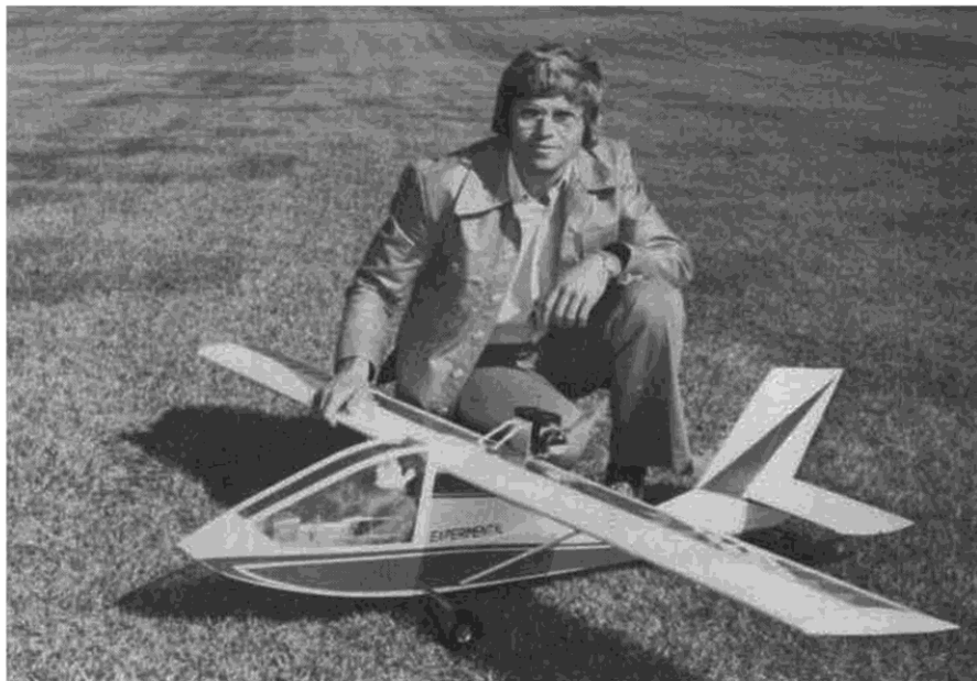
The author and his second "Don Quixote". Slight modifications from the first one are included in the plans. Pusher configuration requires reversing engine operation or L.H. props. See text.
