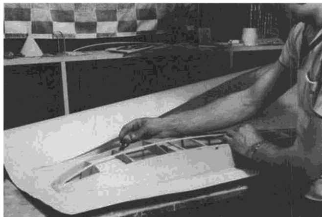
Fuselage is also easy to build on the board because the top is flat. Sides are prebent when doublers are glued on.
