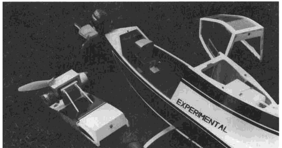
Another view of cockpit area. Everything is quite accessible. Two piece landing gear is installed after fuselage has been finished and painted. Engine braces provide precision thrust adjustments.
