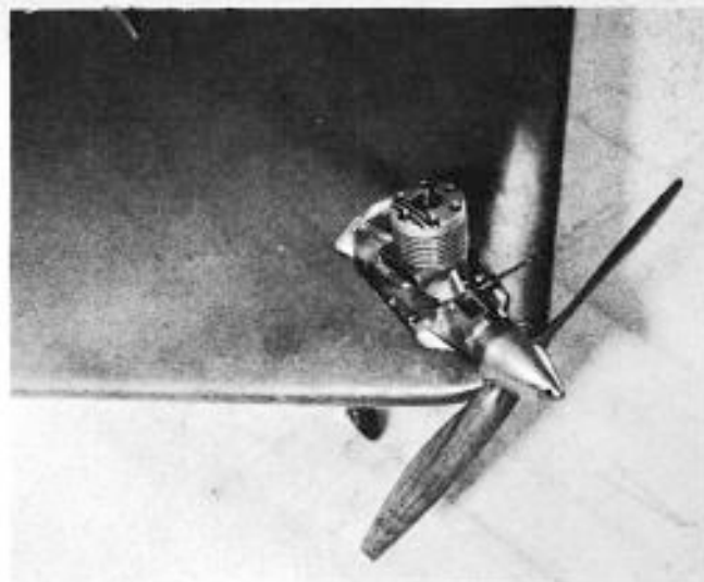
And here we have the end that gives it the momentum to set the new speed records. Latest Super Tigre .15 with high speed prop does the job.
