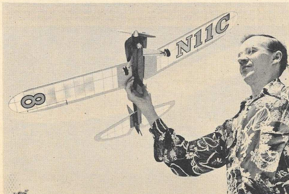
Looks like a long-winged team racer. Good finish, covering, plus applecheek cowls, sheet-metal gear make it look like million bucks. Jobs like this don't come in kits so give yourself building treat.
