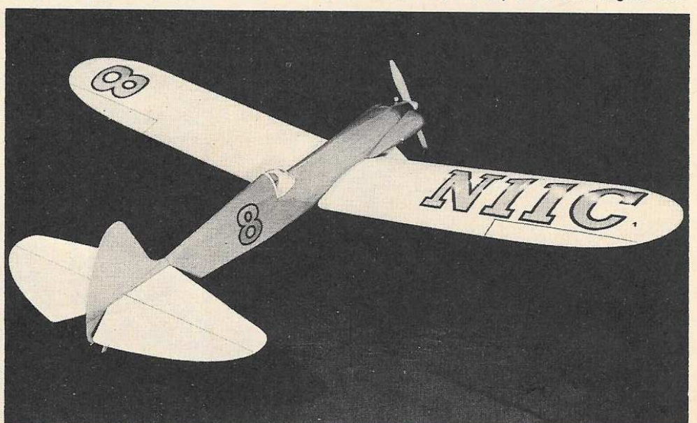
Terrific power of the modern Half-A "mill" is made controllable, flight rendered realistic by use of ample moment arms and "stretched out" lines. Despite all this, construction is not too difficult.
