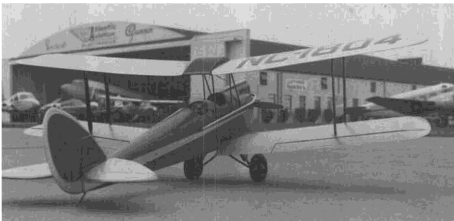
This photo, and the one at the top, were taken soon after completion of the Moth, in 1960. Sprung tailskid was later replaced by steerable wheel. Functional exhaust from Forster .99.
