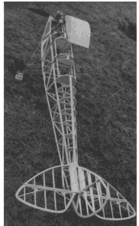
Fuselage and tail framework. Fuselage sheeted with 3/32 balsa. Nylon covering over all.
