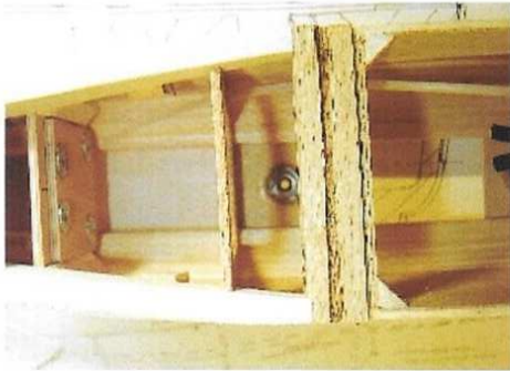
ABOVE LEFT: Front of radio bay before sheeting to form air outlet. ABOVE RIGHT: Rear of fuselage with snakes fitted and skid mount.
