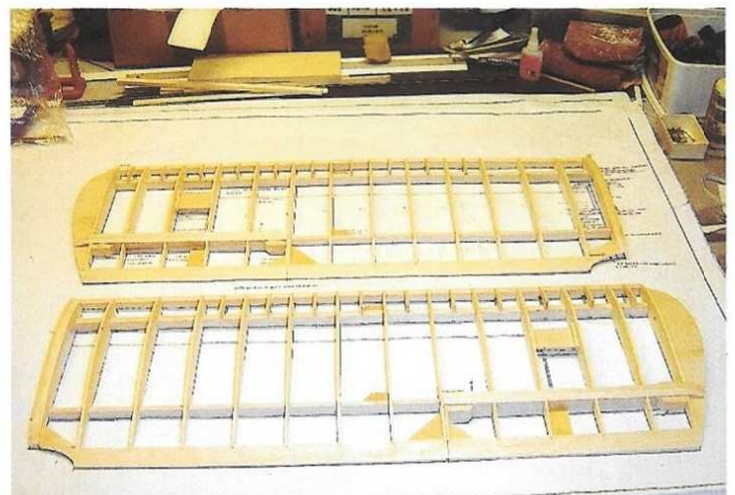
Basic wing structure is light and simple.
