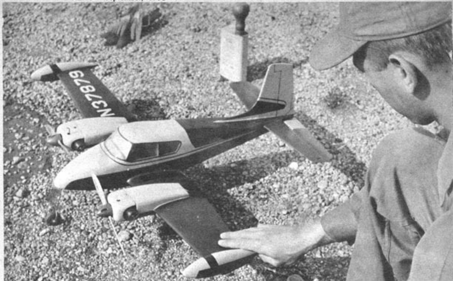
Heads of the twin Webras stick out from the "flat" cowls. For that eye-popping color scheme, sand and sand and do exactly what the man sez.
