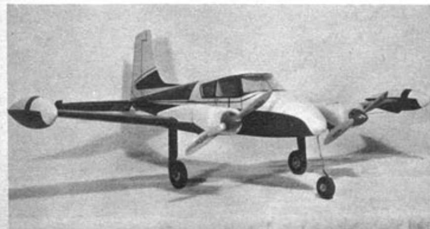
With the exception of lead-outs, needle valves, and other modeling tell-tale details, the only departure from scale is the half inch addition to the gear for prop clearance. Below—pretty, any view.
