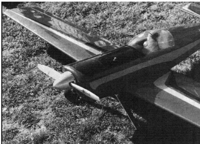
LEFT: Full cowl in place. The split joint for removing just the top is visible. RIGHT: Top of the cowl removed by removing screws on each side that screw into the lower cowl. The two fittings on top of the fuselage are vents for the gas and smoke oil tanks.
