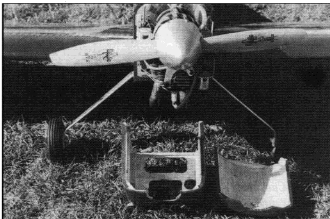
LEFT: By removing four screws in the lower cowl, it can be removed by lowering it around the exhaust pipe extensions. The magneto has been replaced by computerized battery ignition on the left side of the engine. RIGHT: The cowl is totally removed without touching the spinner and prop. The engine is mounted to the fire wall with well nuts and spaced from the fire wall by a piece of 3/4" pine. The carburetor side of the engine gets crowded with throttle linkage, fuel tubing to the carb, and impulse tubing to the smoke oil pump.
