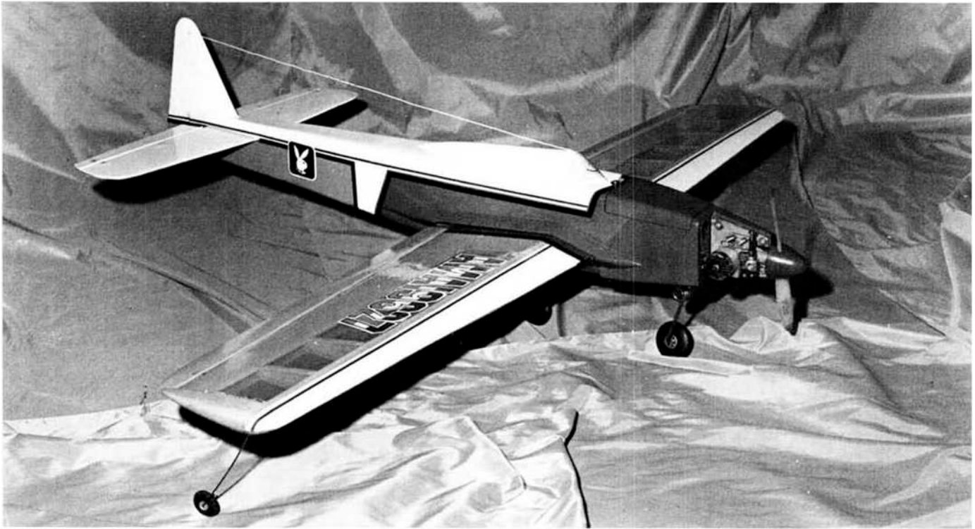
Taking an idea from ukie combat flyers, who have to build quickly, inexpensively . . . and often, John used a diamond airfoil on the wing so that it could be built in one piece, upside down, on the workbench. It has shown no bad characteristics and is stable at slow speeds.
