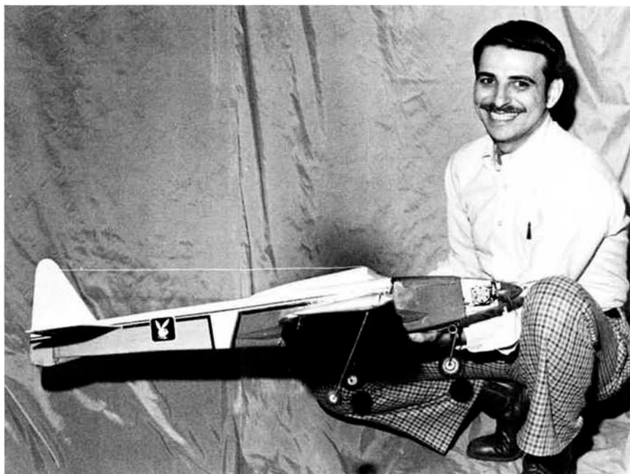
Author/designer John Chapis and the baby Banshee. Note tandem gear and tip wheels. An inexpensive way to practice pattern maneuvers, Bantee uses 3 channels and a .19 engine.
