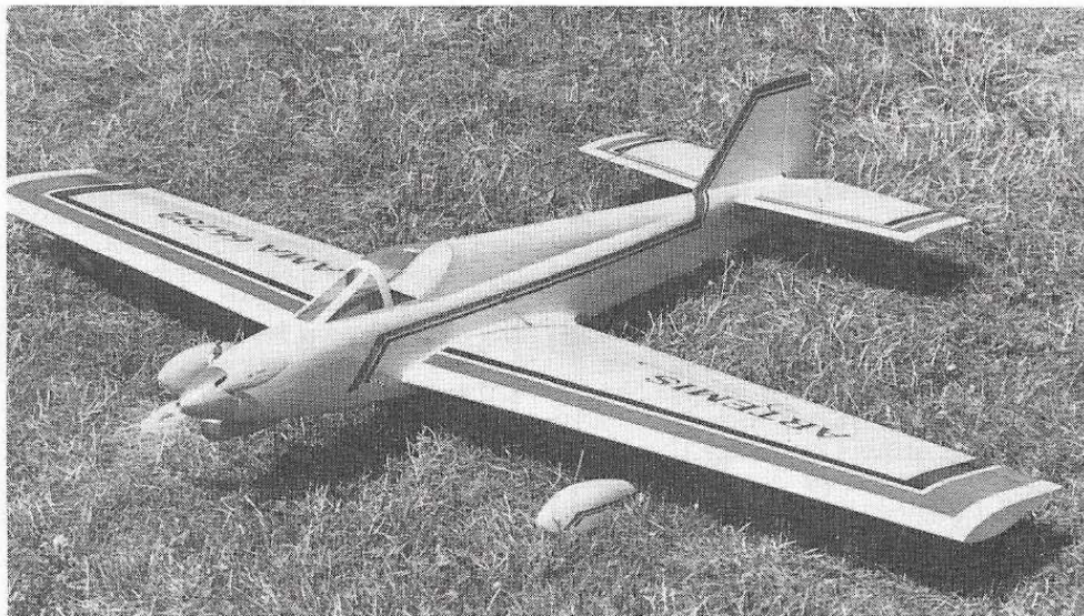
Many of the components are foam—wing, stab cores and the turtle deck. Helps to ease the building chores and get you to the field a little quicker. The clear plastic canopy is from Sig's Kougar .
