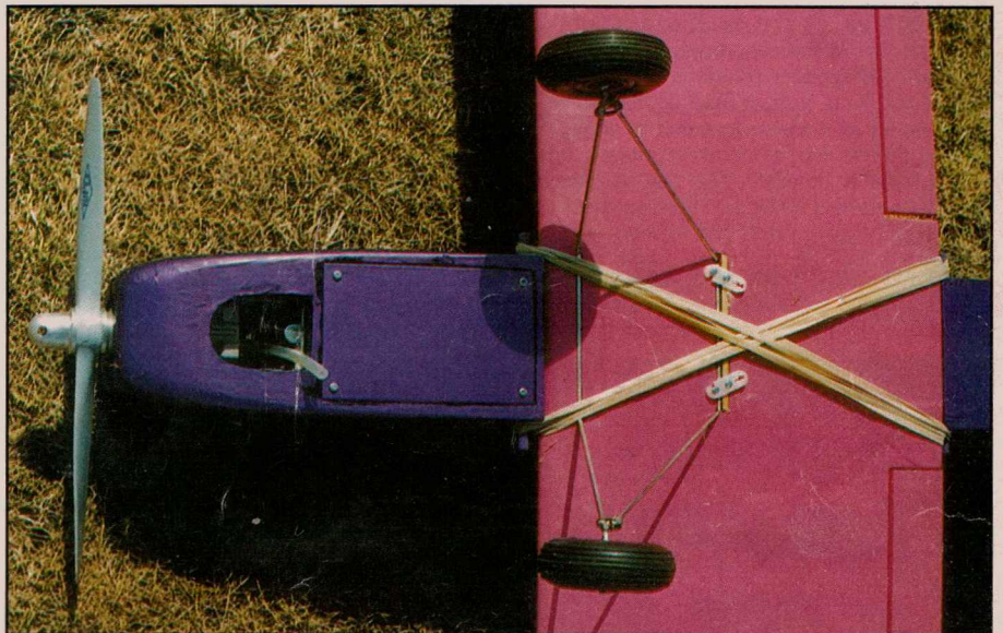
Note u/c fixing arrangement and cowling hatch in this shot; wing is simply banded on.
