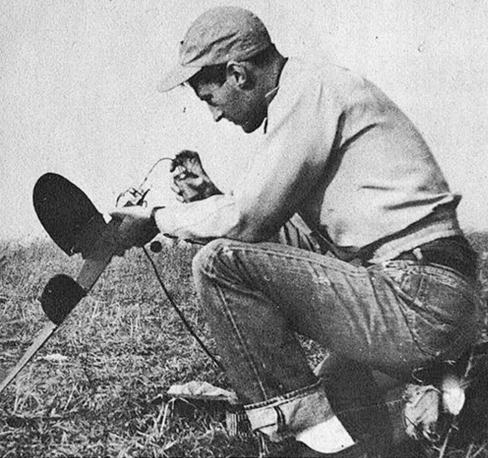
The designer primes the engine of his duo-mono before starting. Developed through a series of models, it is extremely stable, especially in the stalls, and is an excellent windy weather performer.
