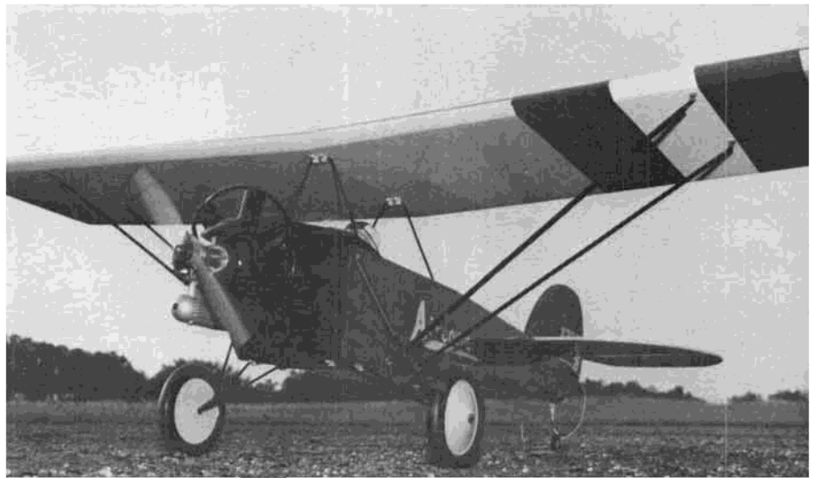
Low angle shot shows simple but functional strut attachment. They could be bolted on permanently, as the plane is relatively small and easy to transport.
