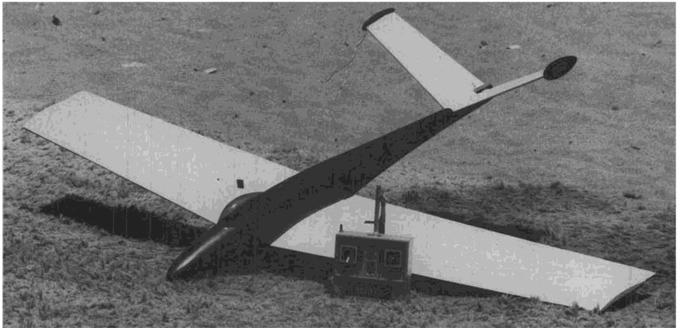
The Afternoon Delite is a fast, maneuverable slope soarer that just might make a good slope racer, with some extra ballast. The model will fly in very light wind, due to its light (25 oz.) weight. Nicely-rounded fuselage is not hard to make, and is well worth the little extra work involved.
